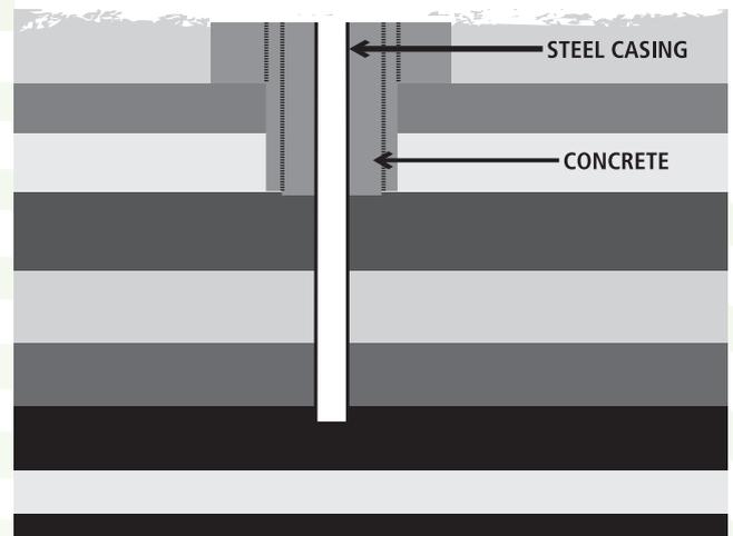
CROSS-SECTION OF A CORE HOLE CASING
