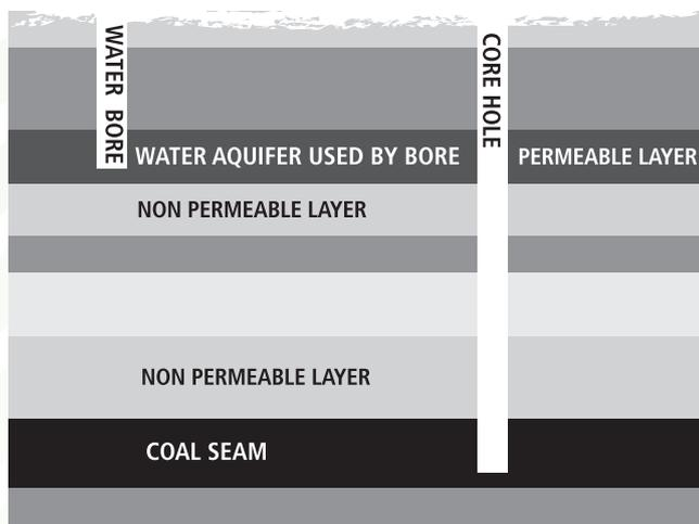
To extract water, using a water bore, drillers drill into an aquifer and pump the water out of this layer. In the Broke and Bulga region, most water bores draw from aquifers that are within 15 metres of the surface, a few draw from deeper depths down to 70 metres. In other areas of the Hunter aquifers used by the community may be more than 200 metres in depth.
